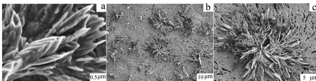
Figure 2. SEM micrographs of self-assembled HTDA-2/DMF at different concentrations and cycles of treatments: (a) 5 wt %, (b, c) 1 wt %/3 cycles.
